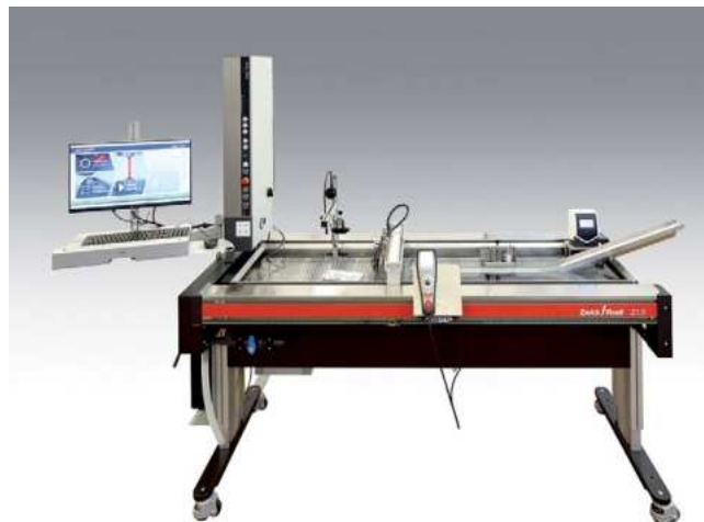
The modular platform enables realistic testing under clinical conditions. It complies with international standards including ISO 10555, DIN EN ISO 25539, and ASTM F623
